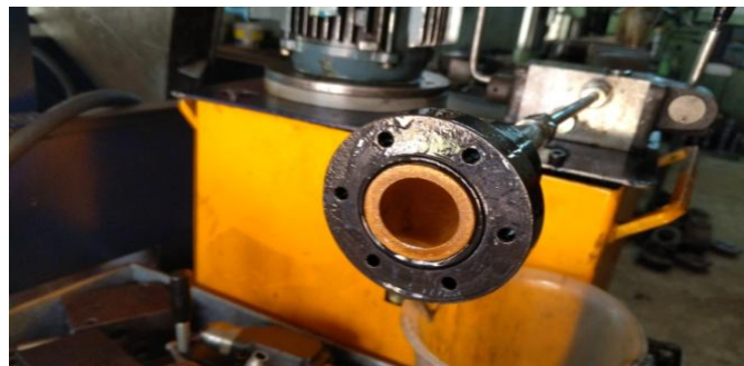
Fig 7.4- Nitrile material seal in filter
