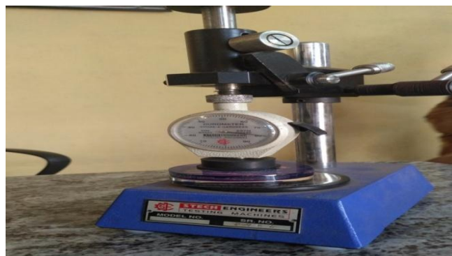
Fig 5.3 – Durometer scale (hardness testing apparatus)
