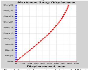
**Chart 4**: Story displacement graph due to wind Y load
