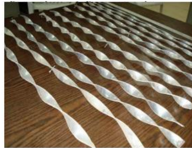
Fig.7 varying width twisted tape [5]
