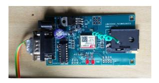
Fig -7: GSM Module
