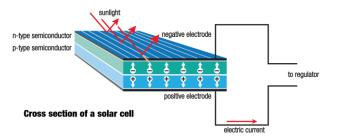
Fig -3: Working of a Photovoltaic cell
