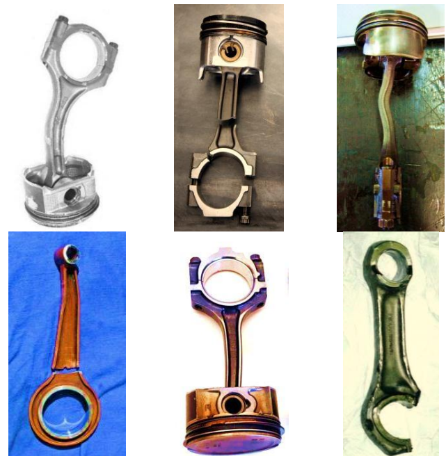
Fig.-1 Various forms of connecting rod failure
