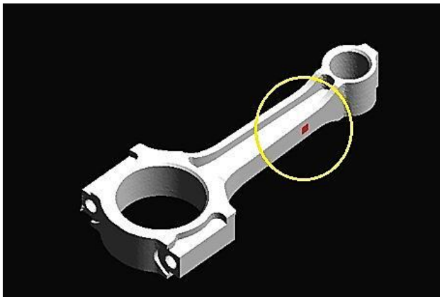
Fig.-3. Ingate location for entering molten metal in die cavity.
