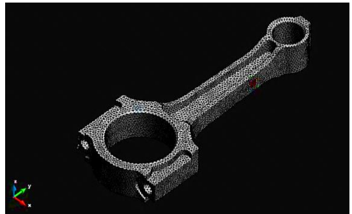
Fig.-2 Connecting rod advanced meshing with 0.2mm element size made in Click2Cast
