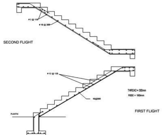
Fig 9 . Reinforcement details of stair case
