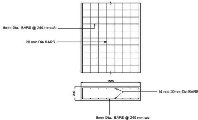
Fig 7. Reinforcement details of shear wall
