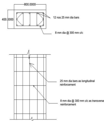
Fig 8. Reinforcement details of column
