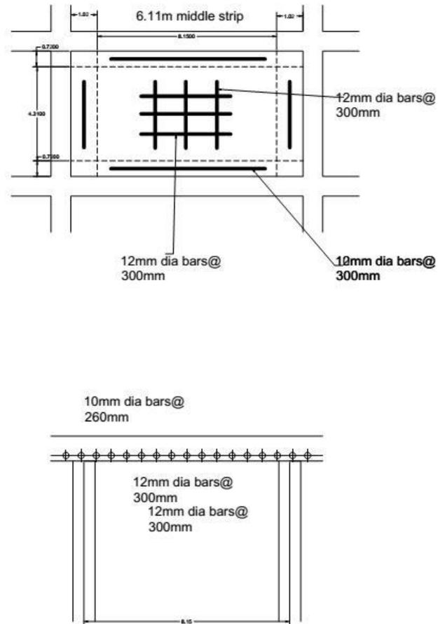
Fig 5. Reinforcement details of two way lab
