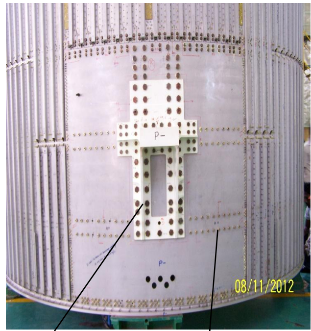
THRUST BLOCK (Steel) ISO GRID PANNEL (Al-alloy)
