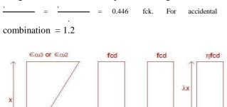
The parabolic-rectangular stress block will be converted in to equivalent rectangular stress block having uniform
