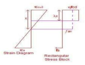
Figure: 4 Stress Strain Diagram for Rectangular Stress Block
