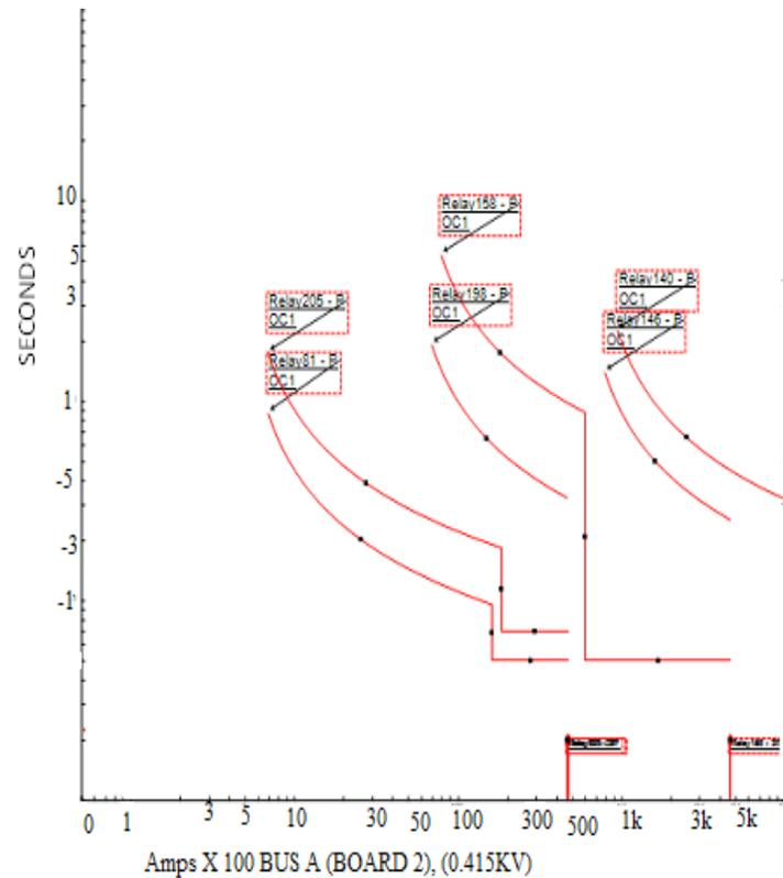
Fig-5: Characteristics of relays
