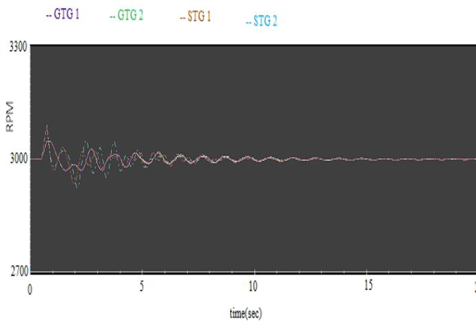
Fig-4: Generator speed
