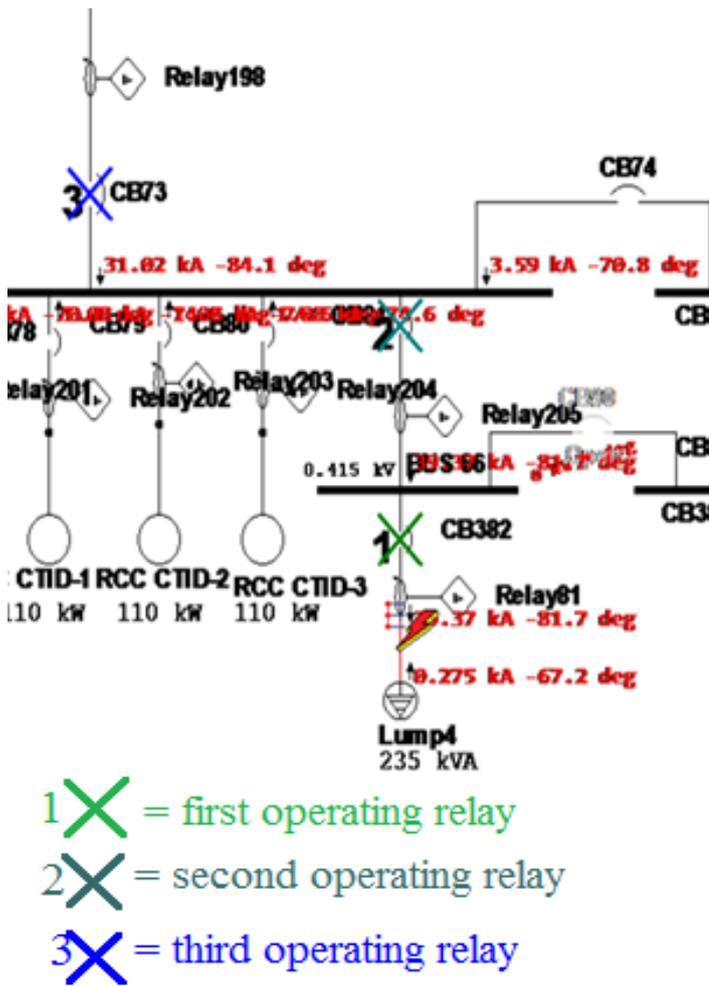
Fig-6: Relay co-ordination of the system
