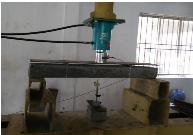
Fig 8.7: Experimental Setup for Conventional RC beams
