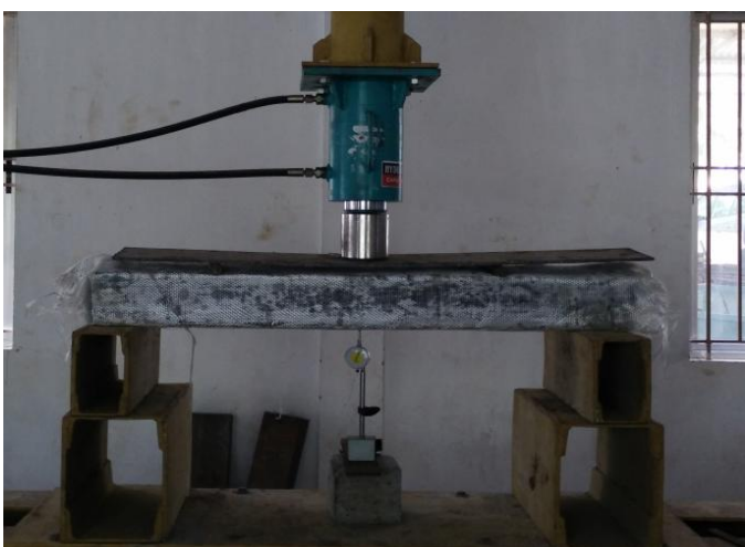
Fig 8.8: Experimental Setup for GFRP Wrapped RC Beams
