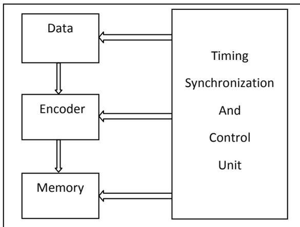
Fig. 2 A simple data encoder block
