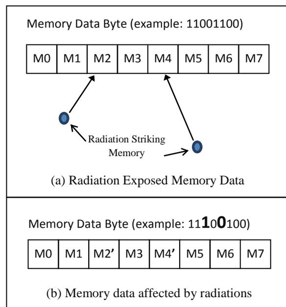
Fig. 1 Soft Error caused in Semiconductor Memory due to exposure to Energy Radiation
