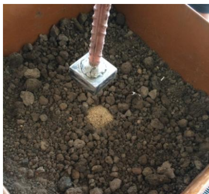
Fig -7: Skirt arranged for testing
