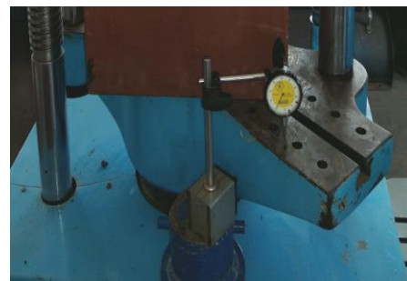
Fig -6: Dial Gauge setup
