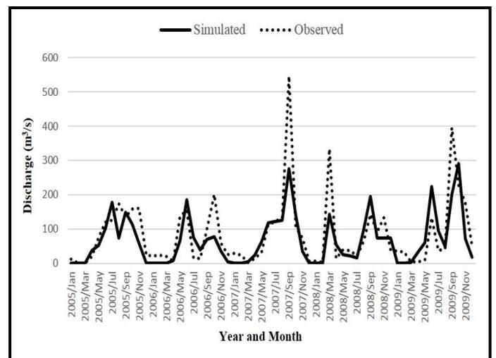
Fig -9: Variation in observed and simulated discharge values on Validation
