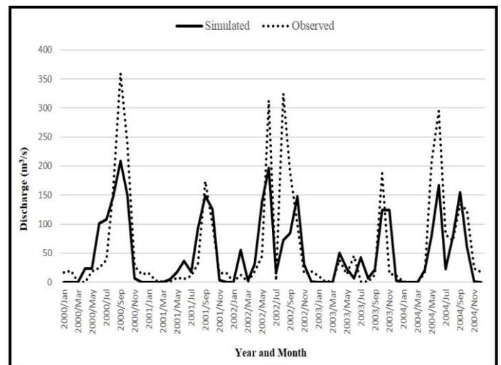
Fig -8: Comparison between observed and simulated discharge values after calibration
