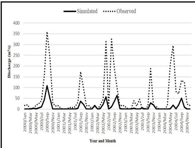
Fig -7: Comparison between observed and simulated discharge values before calibration
