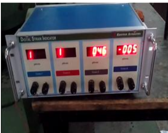
Fig.-11 Strain Reading on Digital strain Indicator for Plate with Relief hole
