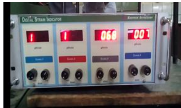
Fig.-9 Strain Reading on Digital strain Indicator for Plate without Relief hole
