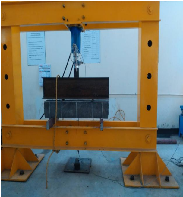
Figure-3 loading frame
