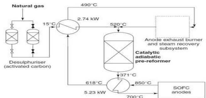
Fig. 2. Pre-reformer system devised for a Siemens 50-kW SOFC demonstration [6].
