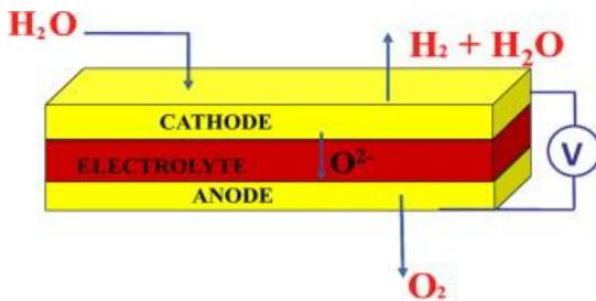
Fig.1. Scheme of a SOFC cell operating under electrolysis mode
