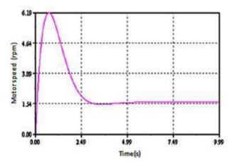
**Chart -2**: Motor speed as a function of time for a load of 3N.
