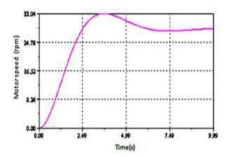
Chart -1: Piezoelectric motor speed without load.
