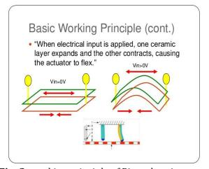
**Fig- 2:** working principle of Piezoelectric motor.
