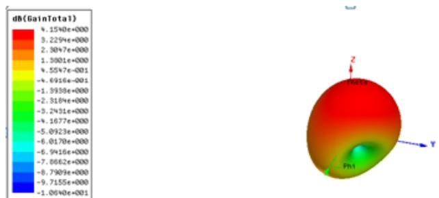
Fig -11: Radiation pattern for 5GHz for two slots PIFA
