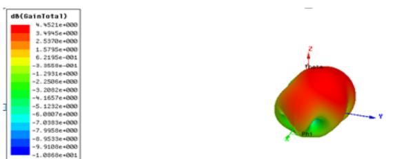
Fig -14. Radiation pattern for 4.8GHz for three slots PIFA
