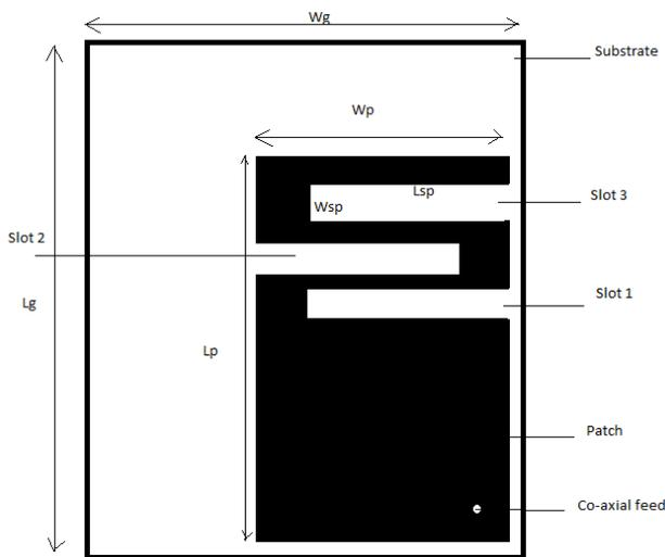
Fig -4: Top-view of PIFA with slots
