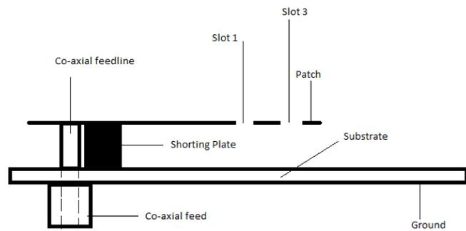
Fig -3: Side-view of PIFA with slots
