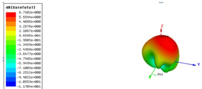
Fig -10: Radiation pattern for 2.3GHz for two slots PIFA
