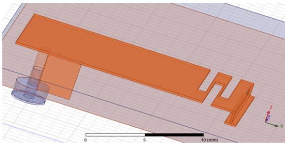
Fig.12 Top view of three slots PIFA
