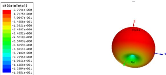
Fig -7: Radiation pattern for 2.2GHz
