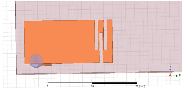
Fig -5: Top-view model of PIFA with slots
