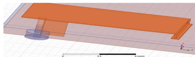
Fig -6: Top view of without slots PIFA
