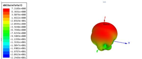
Fig -13. Radiation pattern for 2.2GHz for three slots PIFA
