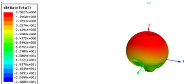
Fig -8: Radiation pattern for 5.5GHz
