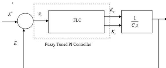
Fig-7 Block Diagram of Fuzzy Tuned PI Controller
