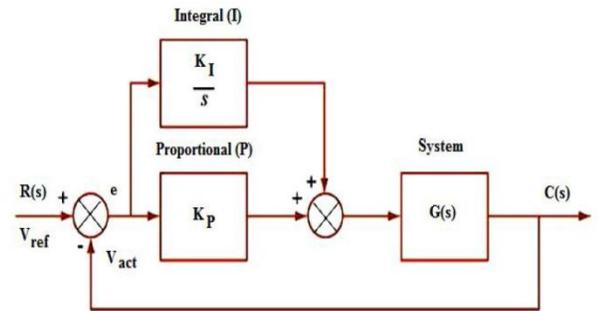
Fig-2 Transfer function model of PI controller
