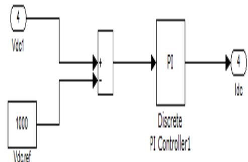
**Fig-3** DC link voltage control using PI controller
