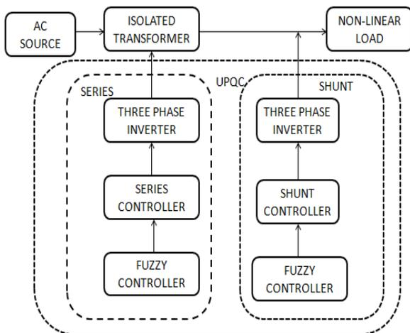
**Fig-4** Block Diagram of Fuzzy Logic Controller
