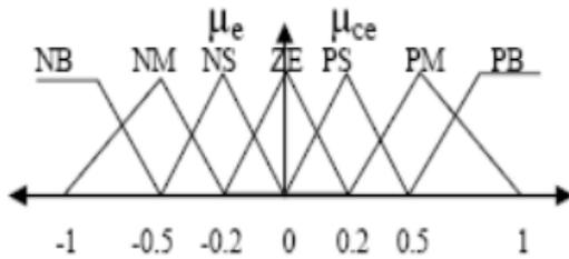
Fig-5 Input Normalized Membership Function
