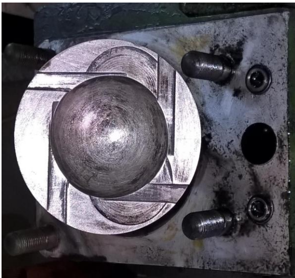
Fig-4: Tangential swirling grooved piston.
