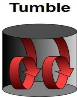
Fig-2: Tumble motion of air in engine cylinder.
