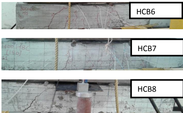
Fig 8: Failure of Hybrid Reinforcement beams
