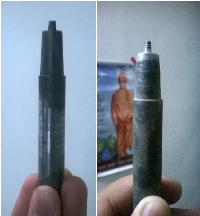
Fig.2-(a) Taper Cylindrical Tool (b) Cylindrical Threaded Tool
