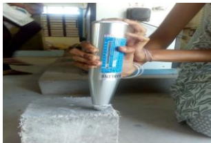
Figure – 1: Rebound Hammer Test
