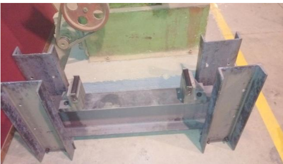
Fig.9 Three-Point Portable testing fixture
