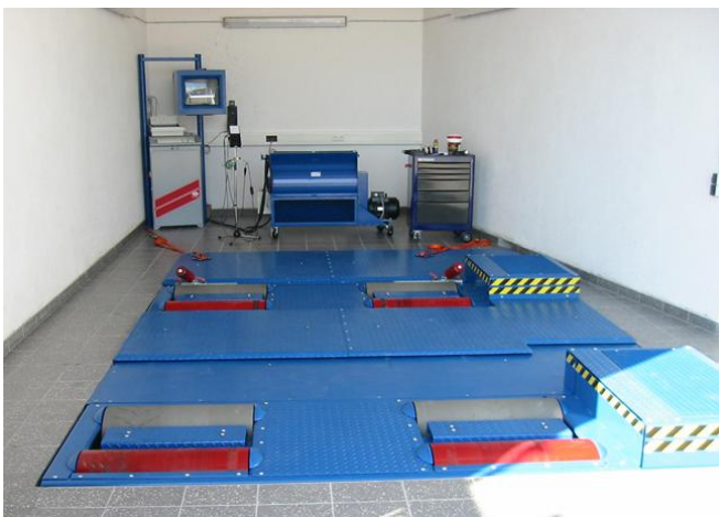
Fig -4: Closed Room Testing (Sample: Road Simulation Test)
