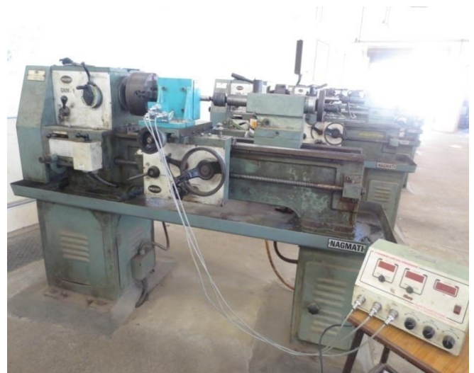
Fig:- 4.1. Lathe Setup with 3-Component Dynamometer
