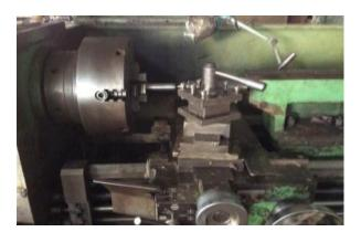
Fig.1: Center drilling of work piece
