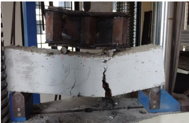
Fig.:12 The failure pattern of doubly beam
