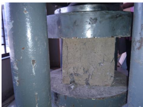
Fig.: 6 Compressive Cube failures
