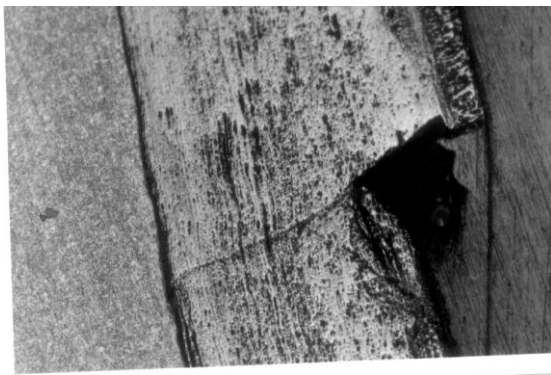
Fig.1.1 Steam side scale; cracking & separation of layer Mag. 50X
