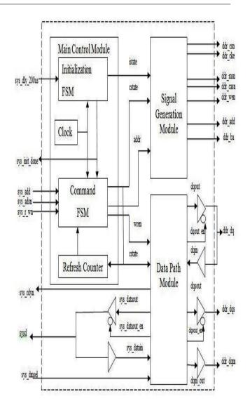
Figure 2Memory Controller Architecture.
