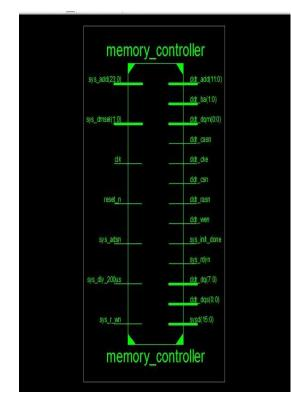
Figure 4Top Level RTL Schematic of the Controller.
