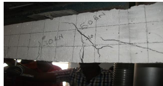
FIG - 6: Failure mode of conventional slab
