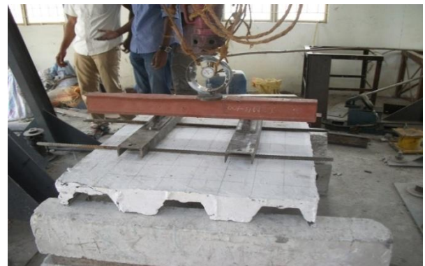
FIG - 3: Test setup of Steel and concrete composite slab
