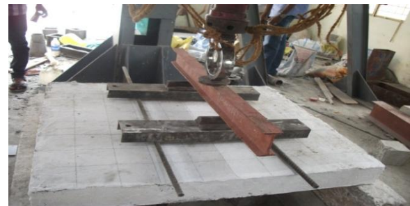
FIG - 2:Test setup for conventional slab
