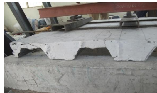
FIG - 7: Failure mode of composite slab
