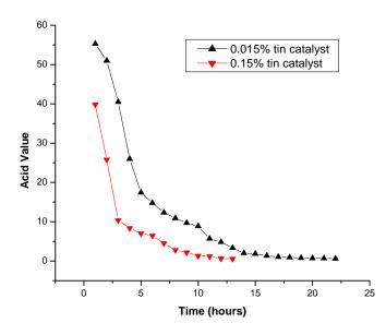
Figure 3 Effect of amount of catalyst on reaction time
