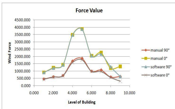
Fig. 18 Comparison of force for both manual and software solutions
