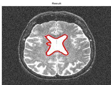
Fig -13:: Segmented noisy image with active contour snake model. Parameters alpha & beta=0.1 kappa & gamma=0.5
