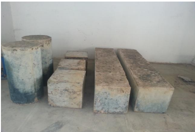
Fig -2: Geopolymer concrete specimens.
