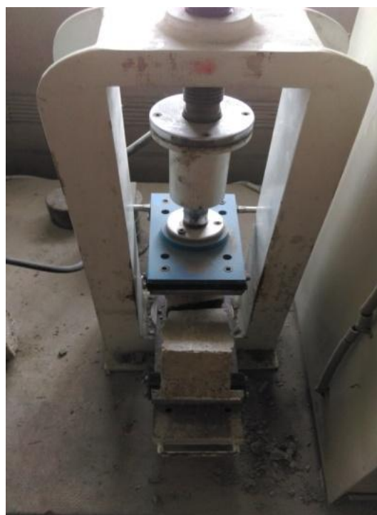
Fig -3: Flexural strength testing machine setup.
