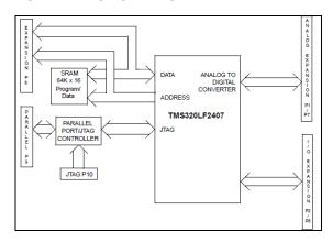
Figure.3 Block diagram OF eZdsp™LF2407
