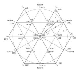
Figure.2 Space Vector Diagram of 3 Level Inverter
