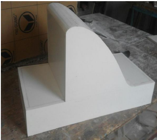
Figure 2.1 (b) Ogee Spillway
