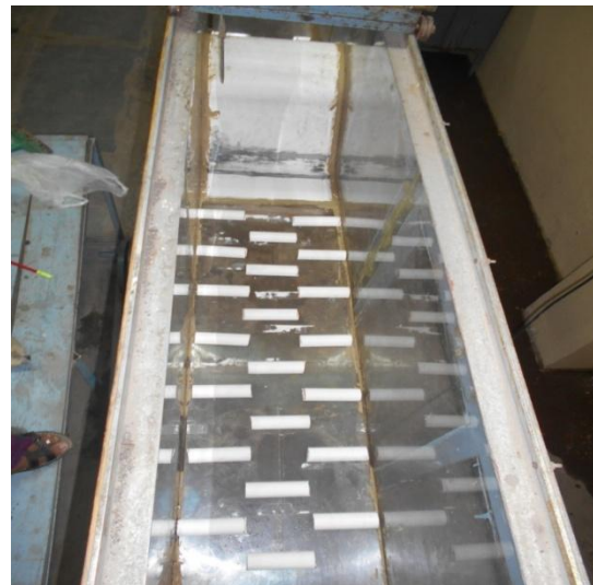
Fig.2.2(b) Staggered Corrugations
