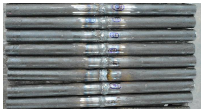
Fig-3: Welded ASTM A106 Pipes
