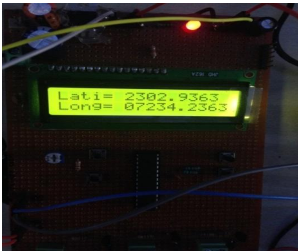
Fig-11: LCD Showing Lati& Long value
