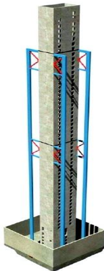
Fig -2: Shear core connected to exterior column via Outrigger truss system (Source- Kiran Kamath, 2014)
