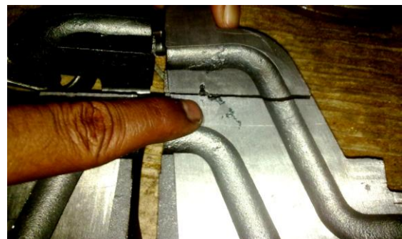
Fig. 6. Internal shrinkage cavity revealed by slicing the component at parting plane
