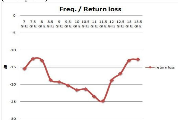
Figure 10: Return Loss for linear profile horn.
