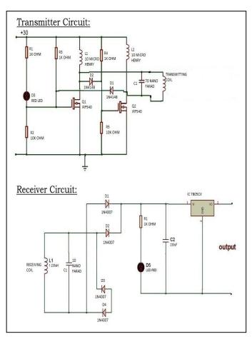
Fig -1: Circuit diagram of the proposed circuit
