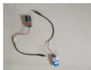
Fig. -3: Power adaptor with 9 V battery.
