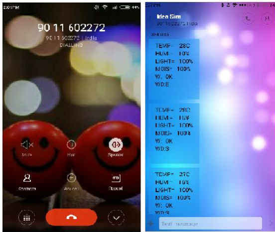
Fig.6 sensed data is sent in message as a response to the call.
