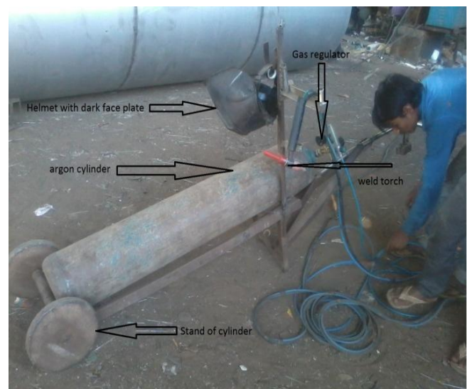
Figure 2. GTAW set up (Courtesy: Apex Engineering, Dediyan, GIDC-II, Mehsana)
