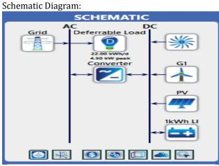
The above Diagram shows the connection of hydro power plant along with other sources of power in Green Building, which are solar power (PV cells), Wind turbine, Battery banks and the Grid.
