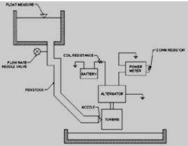
The layout of a common Pico hydro power plant is given by the above figure. The various components used in Pico hydro power plant are the reservoir, penstock, nozzle, turbine, alternator, battery and net meter. Reservoir is used to store the water and is supplied to the turbine through the pen stock through the vent. The flow of water is controlled with the help of valve. The turbine rotates due to force of water which due to which the turbine rotates.
