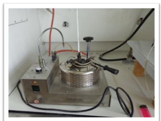
Figure 2.5. Automatic Pensky-Martens Tester
