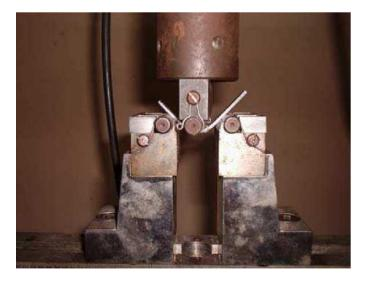
Fig -2: Loading arrangement for flexural test
