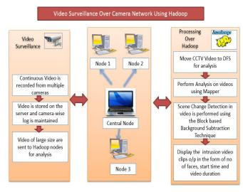
Proposed method uses an Opencv tool to capture camera images and detect intrusion using comparison - block based motion object detection method. As soon as the comparison is done and an intrusion is found, it saves the streamed video on server. After that video analysis is performed using Hadoop technology.
